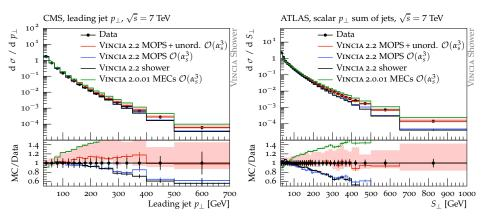
VINCIA 2.2 and VINCIA 2.0.01 predictions compared to ATLAS and CMS data. Predictions are rescaled to the experimental inclusive one-jet cross section. ME corrections are applied for  $\leq$  3 emissions. The red band is obtained by varying the effective scale in non-shower events by factors of two.
