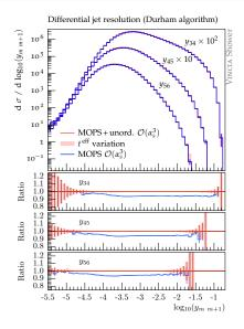
VINCIA predictions for jet resolution measures  $y_{m\,m+1}$  (Durham) for lepton collisions. ME corrections are applied for  $\leq$  3 emissions. The red band is obtained by varying the effective scale  $t^{\rm eff}$  [GeV] in non-shower events by factors of two.
