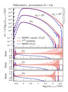
VINCIA predictions for jet resolution measures  $d_{m\,m+1}$  (longitudinally invariant  $k_{\perp}$  jet algorithm with R = 0.4) for hadron collisions. ME corrections are applied for  $\leq 3$  emissions. The red band is obtained by varying the effective scale  $t^{\rm eff}$  [GeV] in non-shower events by factors of two.
