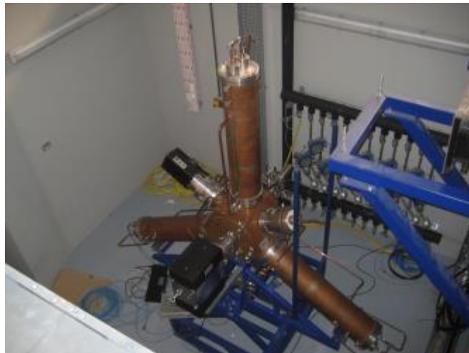
ALBA Cavity inside the Bunker
