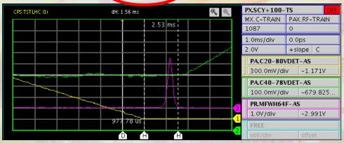
>1 ms error in a 2 ms time window to make a valid measurement for LHC at 26 GeV/c # FWS at C1190 with v = 15 m/s
