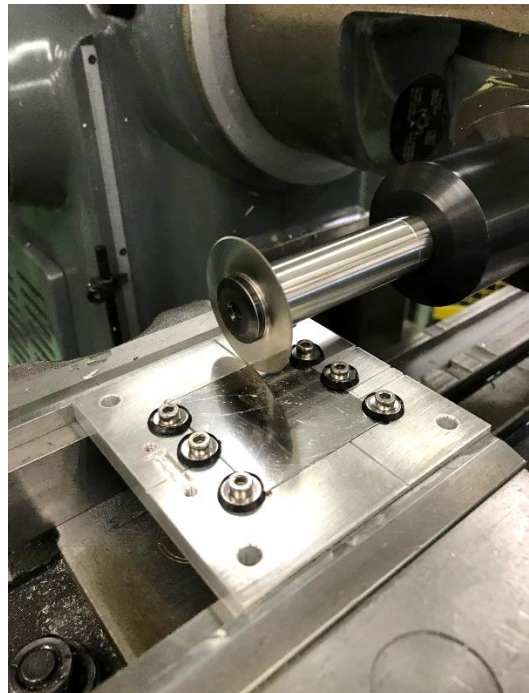
Figure 24 On the left the cutting scheme of the coated samples. Sample dimensions before coating 53 x 53 mm 2 . On the right Samples cutting set-up at INFN.
