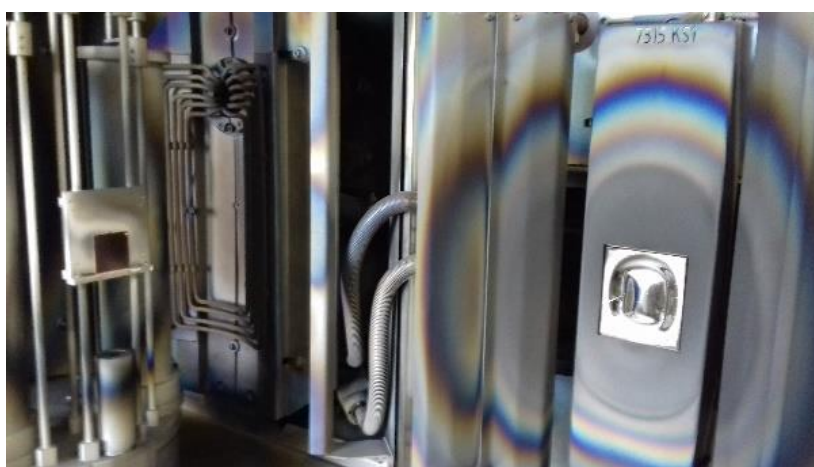
Figure 28 Open deposition chamber with Nb target (right) and installed Cu substrate (left).
