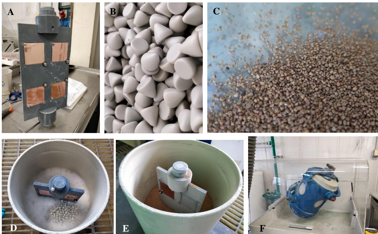
Figure 17 Pictures of the Set-up of the tumbling polishing procedure. A) Sample holder, B) Allumina embedded in ureic resin, C) Coconut powders, D) Tumbling barrel filled with alumina media and Rodastel30 bath, E) Tumbling barrel filled with coconut powders, F) Turbula tumbling machine
