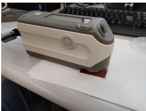
Figure 3 Set-up for the Reflectivity characterization
