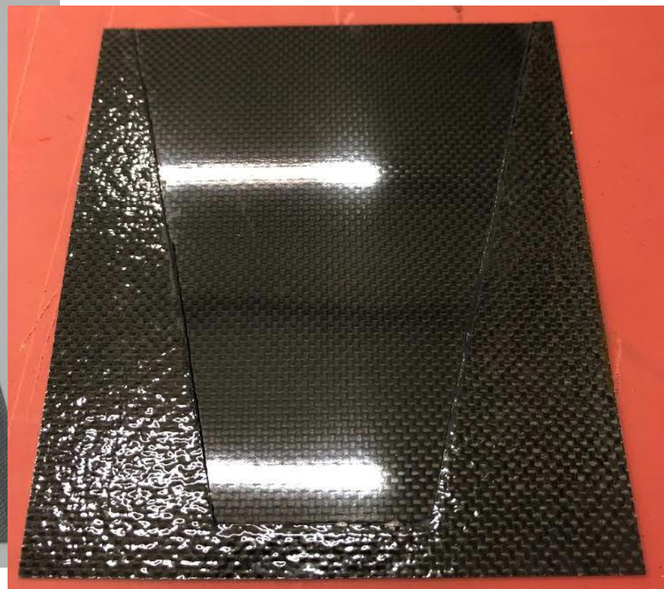
new carbon fibre envelop (plies with woven fibres) 15 of these to be produced
