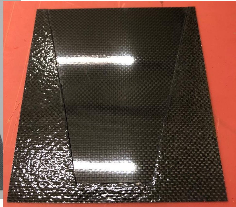
new carbon fibre envelop (plies with woven fibres) 15 of these to be produced
