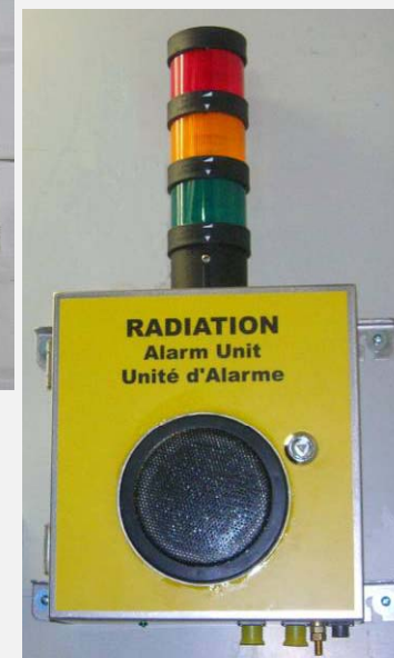
Radiation Alarm Unit (RAMSES)
