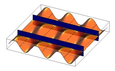
Metallic walls may be inserted where  $E_y = 0$ without perturbing the fields. Note the standing wave in *x*-direction!
