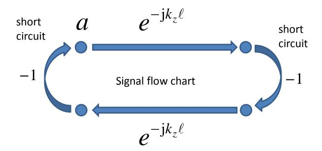
Eigenvalue equation for field amplitude *a*:
