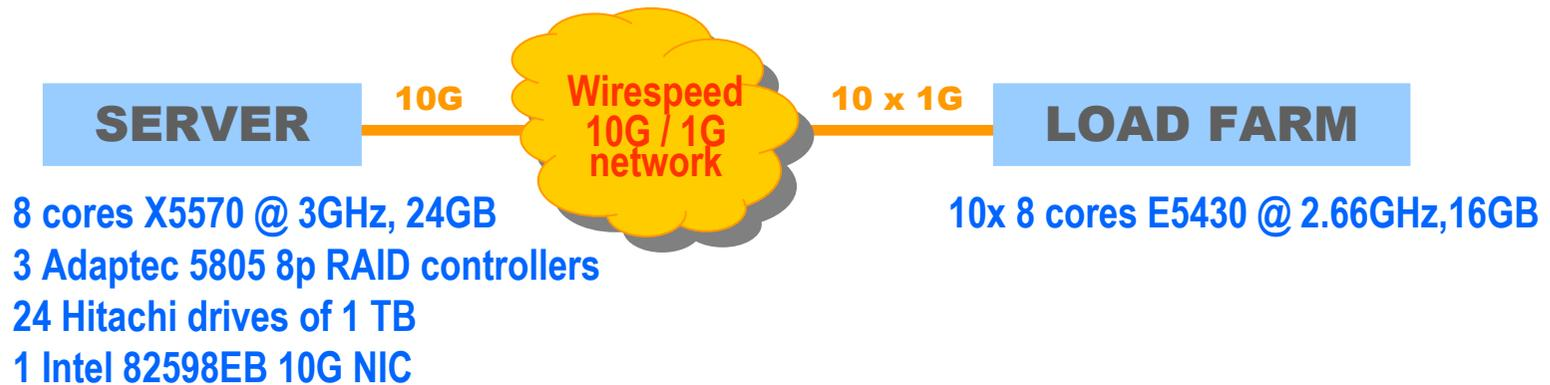
This setup represents well an elementary fraction of a typical large hardware installation and has basically no bottlenecks:
