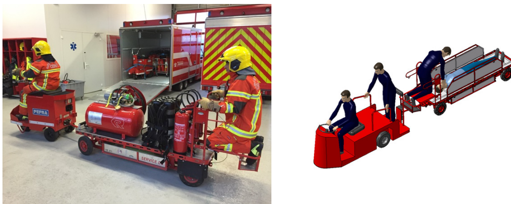
Figure 14 — The tractor with CAFS, spare SCBA, and other equipment (left). The tractor being used to transport an unwell person.
