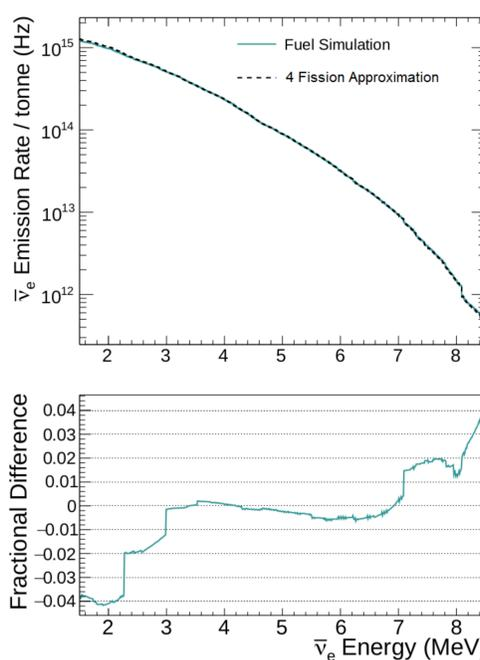
Figure 2: Comparison between the 4 fission spectra approximation and the full reactor calculation. the total integral over detectable anti-neutrinos is consistent to within 2%
