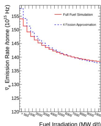
Figure 3: Total detectable anti-neutrinos predicted by the fuel simulation and 4 fission spectrum approximation converge as fuel time in reactor increases
