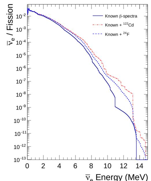
Figure 4: Difference between  $^{239}\text{Pu}$  anti-neutrino emissions calculated from known beta-spectral data only and two theoretical spectra where missing data has been filled in with spectral data from  $^{24}\text{F}$  and  $^{122}\text{Cd}$
