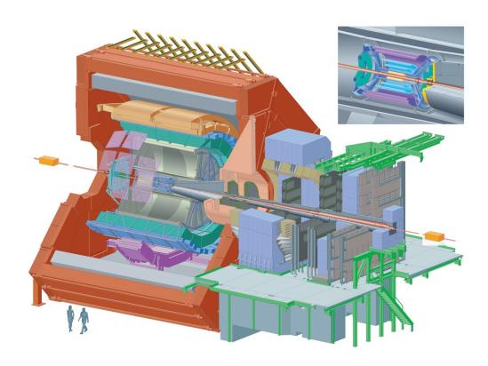
Specificity: low-momentum tracking and particle identification in a high-multiplicity environment
