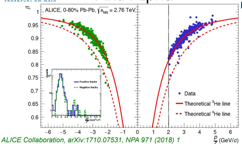
TOF  $\beta$  vs p/z after pre-selection of  $3\sigma$  in TPC shows clear separation  $\rightarrow$  Cut on Alpha needed to suppress contamination
