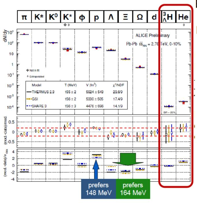
Both hypernuclei and molecular states (deuteron, <sup>4</sup>He) are well described by a thermal model with a temperature around 156 MeV. Hypernuclei are dominated by light quark properties
