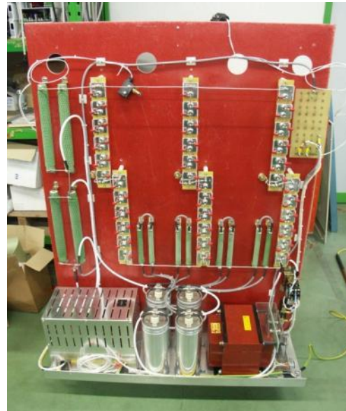
HV Power Supply
