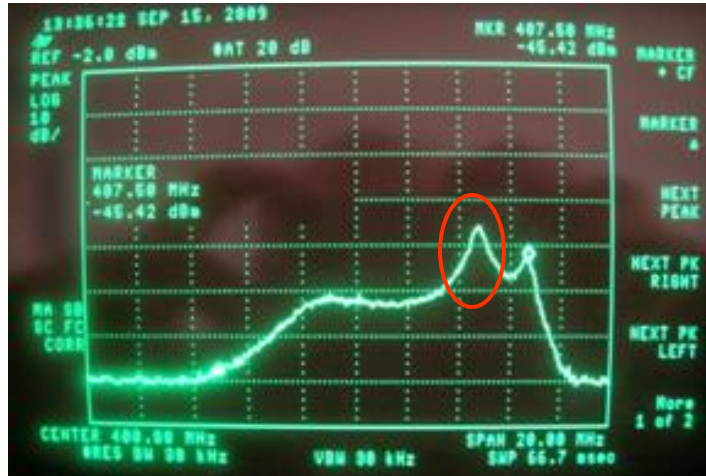
Klystron low signal sweep f_0 \pm 6 MHz
