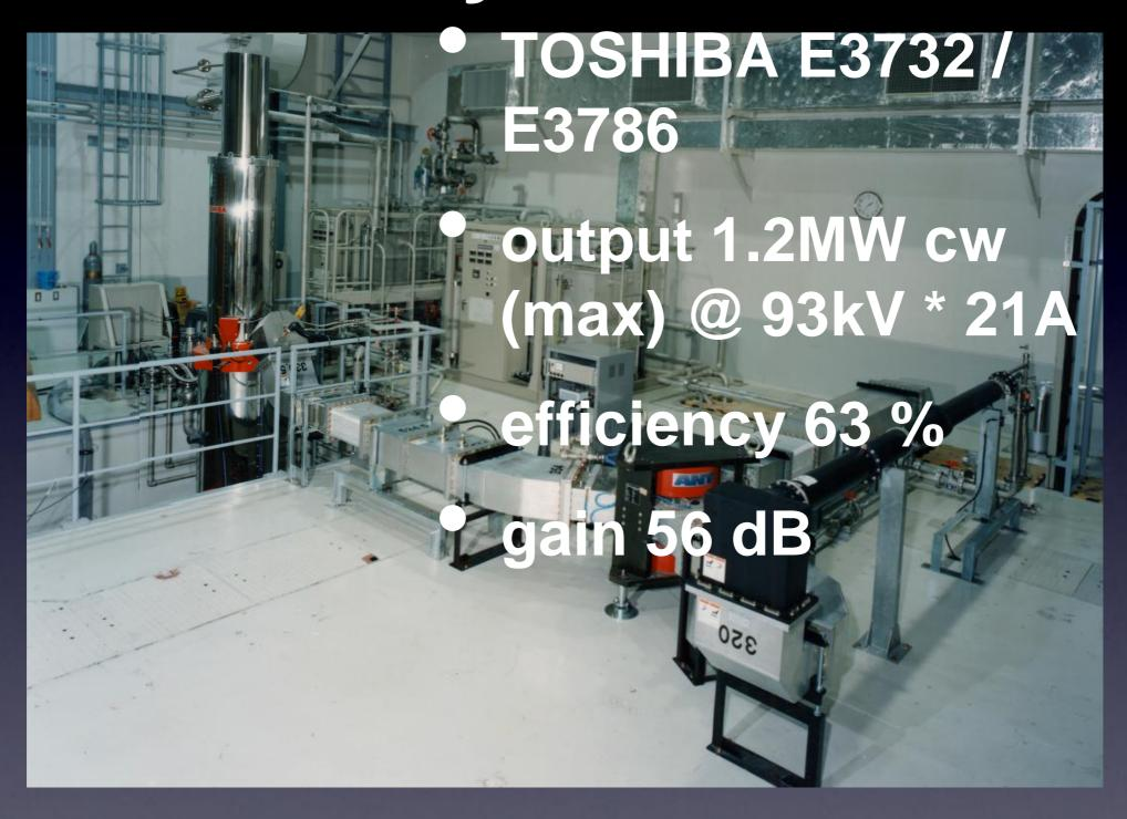
Operation: 300 ~ 700 kW / klystron
