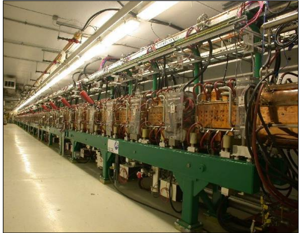
The 805 MHz CCL is composed of four sections.
