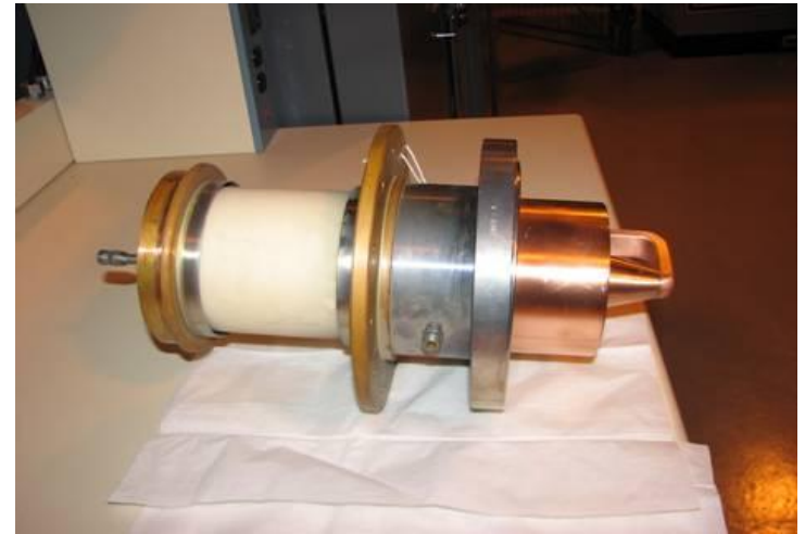
FAILED BOOSTER C1 COUPLER
