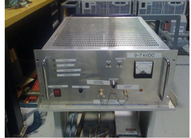
Lambda 202A: 0 – 10kV 2000J/s Average charging rate 2200J/s Peak charging rate → Charging Current = 0.44A
