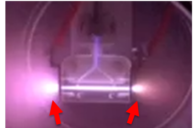
Almost constant plasma density outside the capillary of the order of 10^{15} \text{ cm}^{-3}
