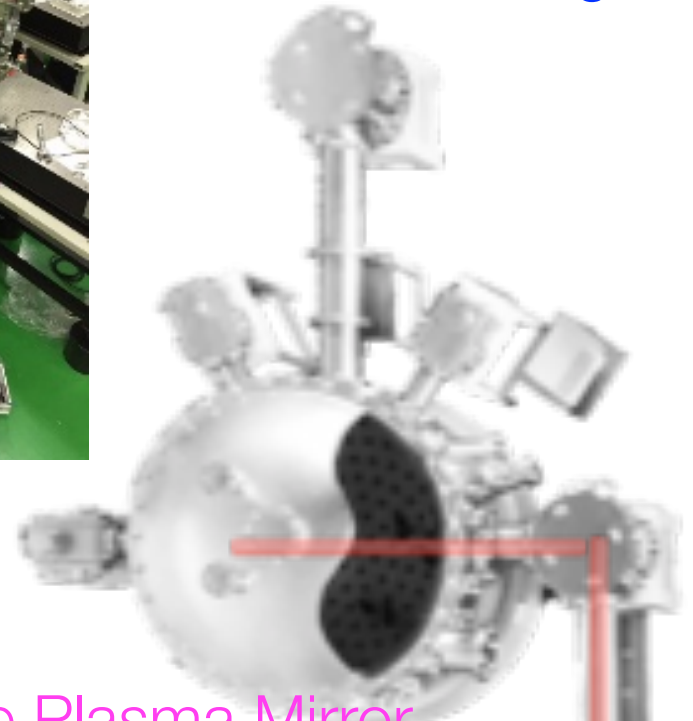
Solid Target Interaction Chamber F/1 - F/5 focusing, 1 beam, PM option
