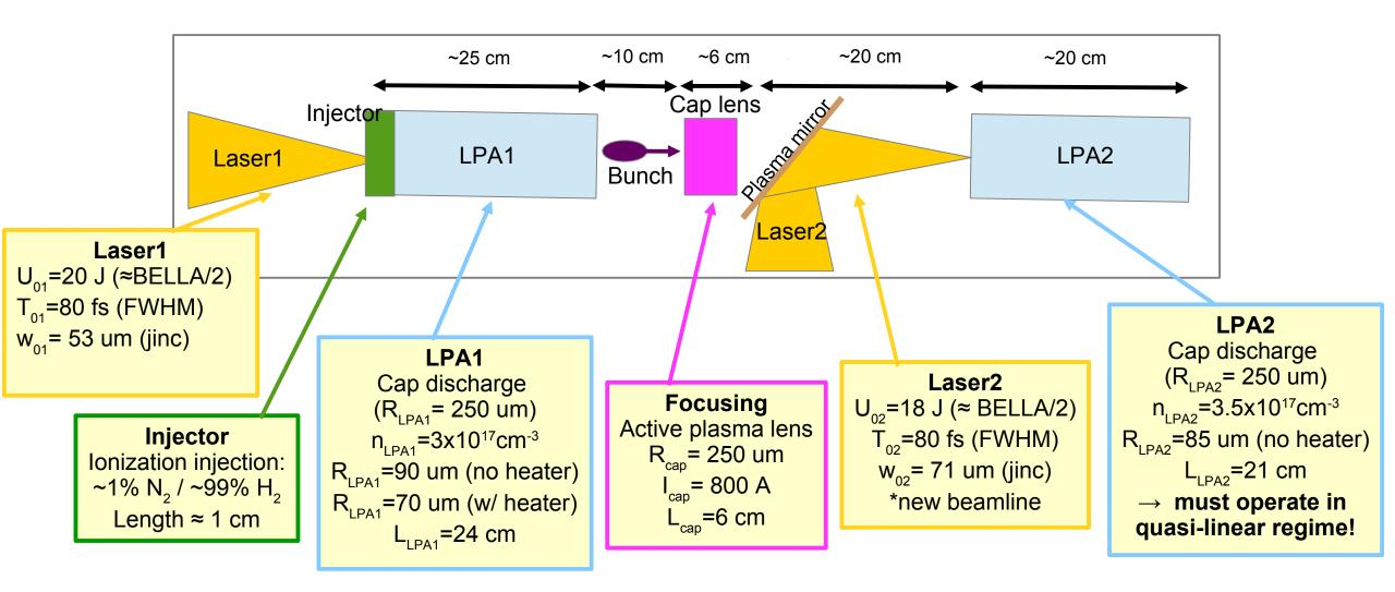
→ Plasma mirror realized with liquid crystal film (small thickness, negligible impact on bunch emittance) [collab. with OSU]
