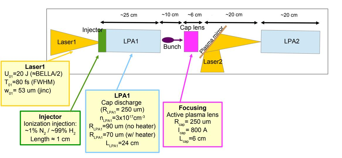
→ Plasma mirror realized with liquid crystal film (small thickness, negligible impact on bunch emittance) [collab. with OSU]
