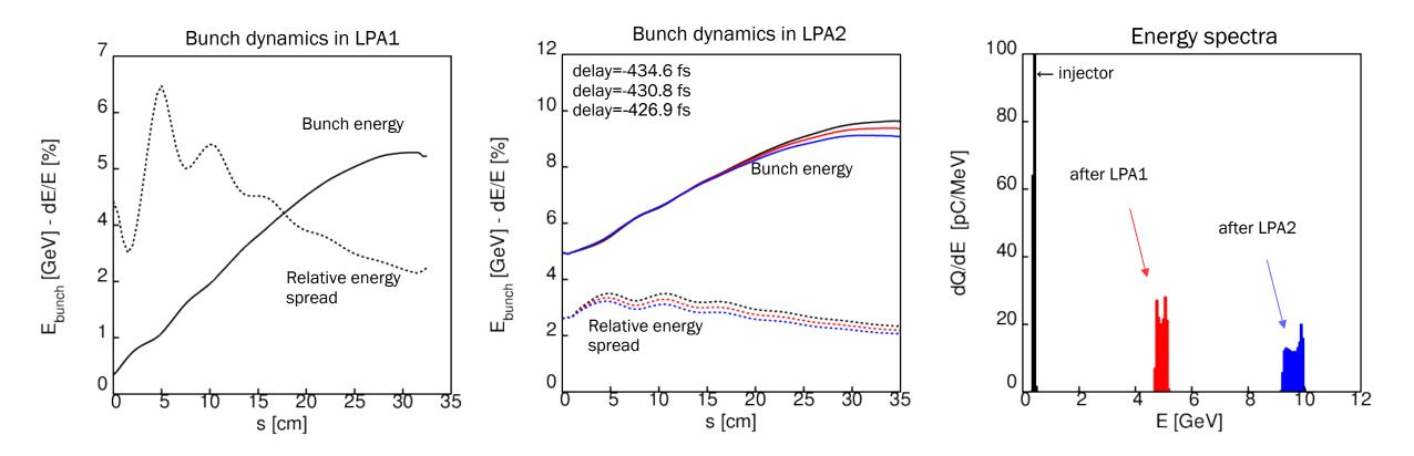
$\rightarrow$  Producing and maintaining low energy spread is key element for 100% bunch capture
