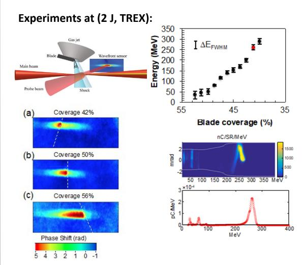
H.-E. Tsai et al., PoP **25**, 043107 (2018) K. K. Swanson et al., PRAB **20**, 051301 (2017) **15**  Development of key technologies for multi-GeV staging with BELLA already underway II: study of plasma plumes and focusing of 1.7 GeV beams with an active plasma lens
