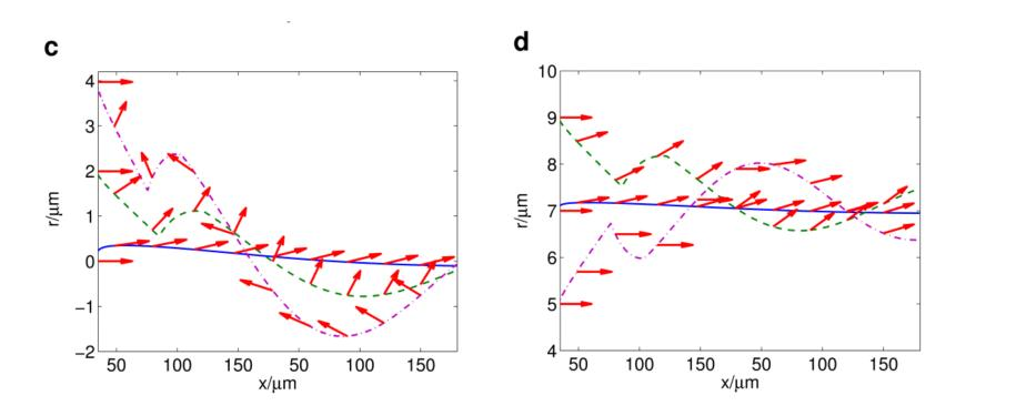
LEFT: in the Gaussian case, the electron spins oscillate incoherently at high frequencies and lose their initial spin orientations instantly
