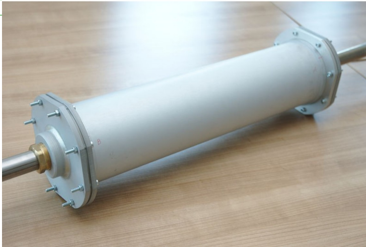
Run 3 chamber, R \approx 7 cm No o-Ps production medium 2 days of measurement
