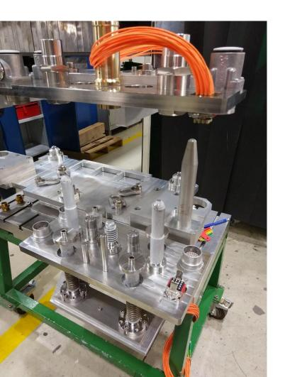
All connections are centralized on a separate plate with independent coupling.
