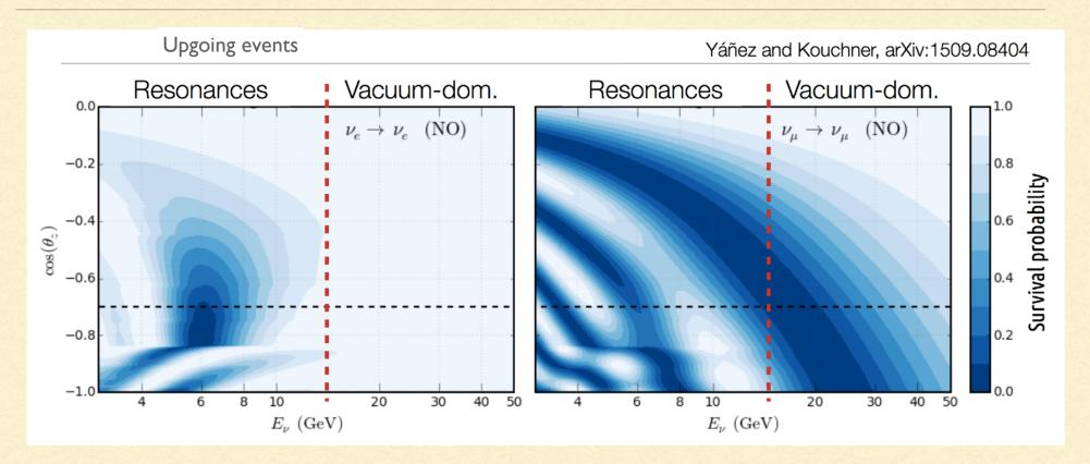
Track(cascade)-like events at neutrino energy 20 GeV have median angular resolution of 10° (16°) and energy resolution 24%(29%).
