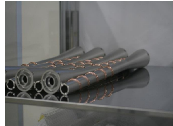
Coupler tips inner part showing cooling channels
