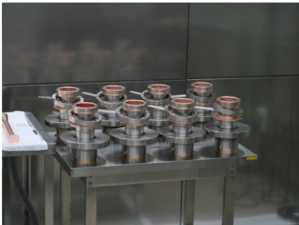
Outer conductor including cavity flange (including cooling)
