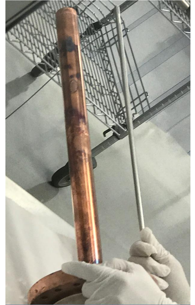
Inner conductor after ultrasonic cleaning
