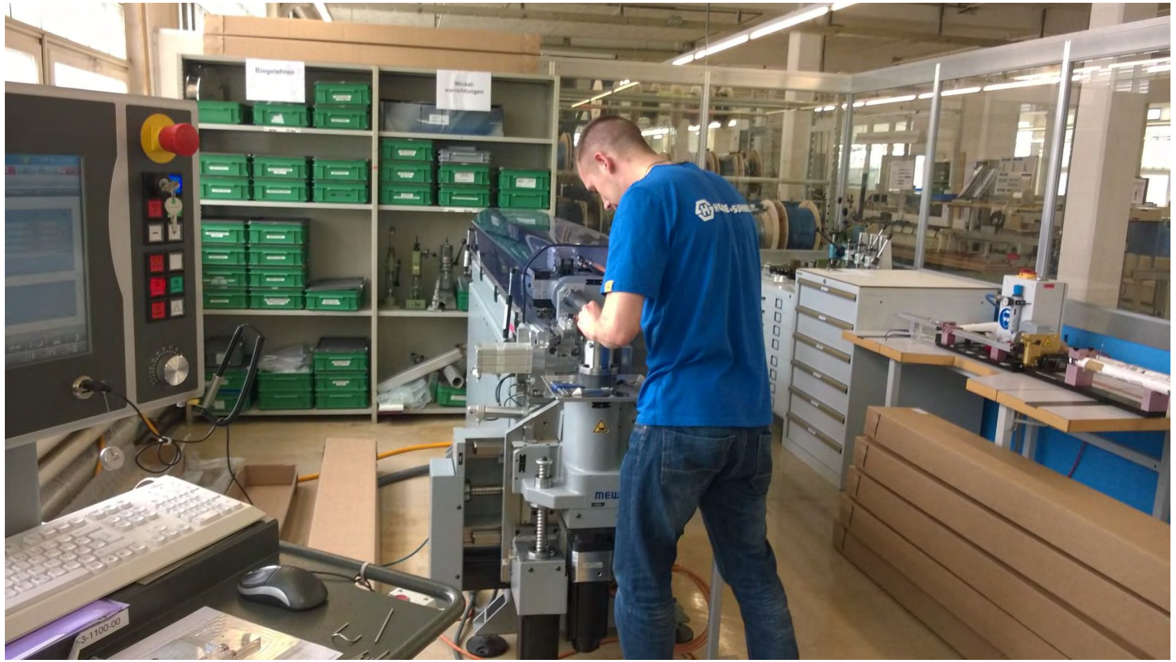
CNC Bending machine at Huber & Suhner
