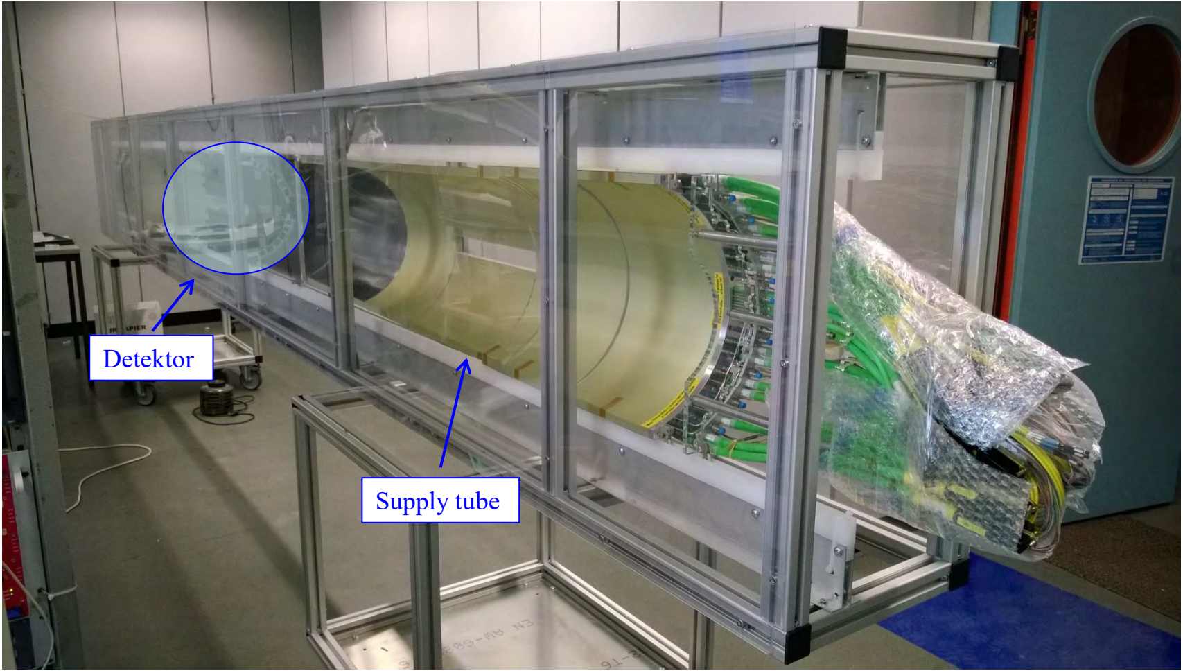
Completed BPIX detector halfshell
