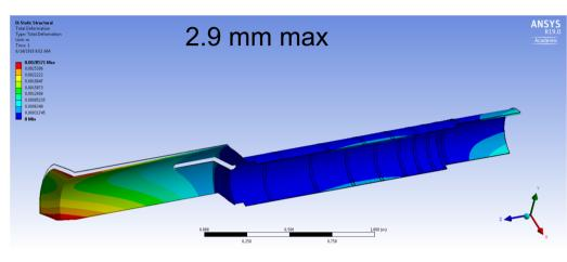
1mm thick CF laminate, 4 wheels, mass of 5kg per double-dee, no mass for services
