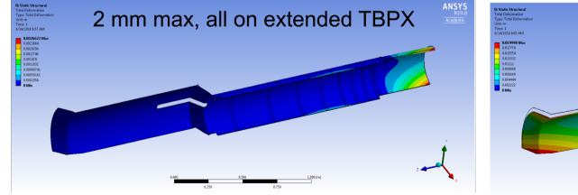
3mm thick CF laminate, 4 wheels, mass of 5kg per double-dee, no mass for services
