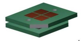
The female pigtail shown connects to all port cards in this cartridge and exits out to service cylinder to make the mating connection
