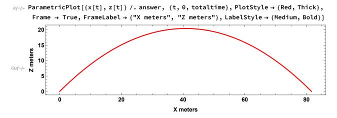
Let's imagine that there is a wall at x = xwall < 80 meters. Then the time the ball hits the wall is
