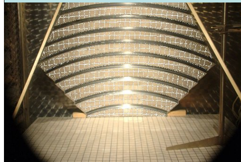
Fiducial net reflection at the first mirror prototype
