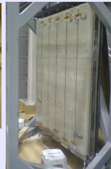
Water panels 6 layers of 25 mm (~ 400 kg)
