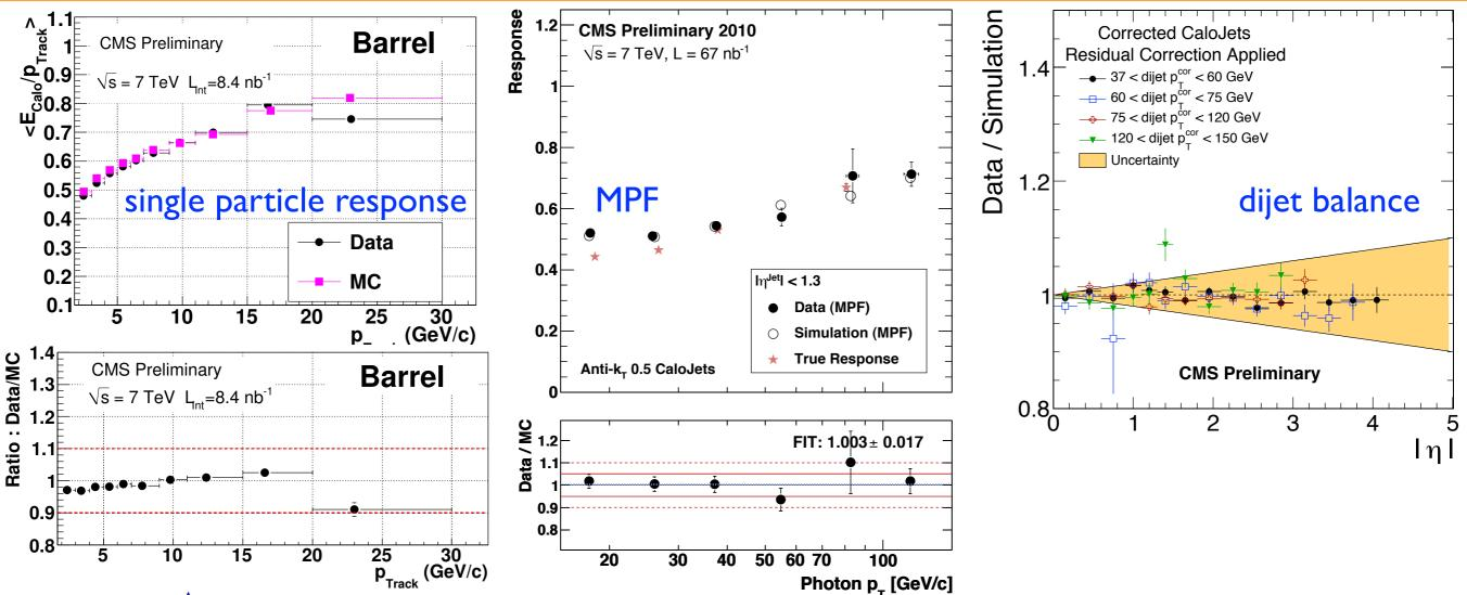
Preliminary measurement of the single particle response indicates that the data vs MC agreement is better than 3% in the barrel.
