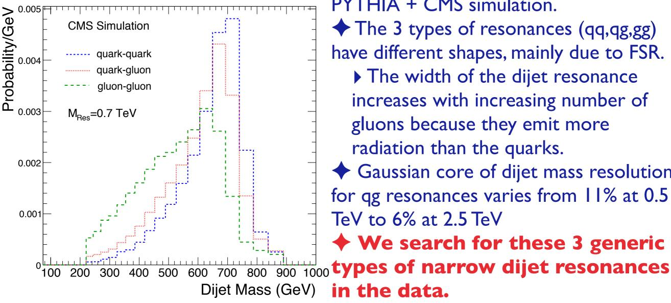
Resonance shapes are produced with PYTHIA + CMS simulation. The 3 types of resonances (qq,qg,gg) have different shapes, mainly due to FSR. The width of the dijet resonance increases with increasing number of gluons because they emit more radiation than the quarks. Gaussian core of dijet mass resolution for qg resonances varies from 11% at 0.5 TeV to 6% at 2.5 TeV We search for these 3 generic
