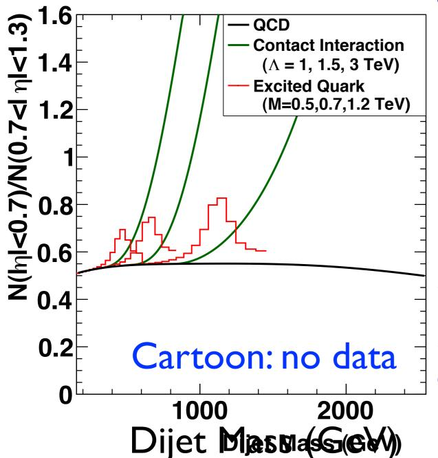
• Quantifies the **centrality** of the dijet angular distribution at a given dijet mass. both leading jets are required to lie in the same  $\eta$  range. "t-channel" scattering for QCD vs "schannel" for most new Physics models approximately flat vs dijet mass for QCD. rises vs dijet mass for contact interactions. "bumps" in dijet mass for dijet resonances. The analysis of the dijet angular distribution is complimentary to the spectrum analysis.
