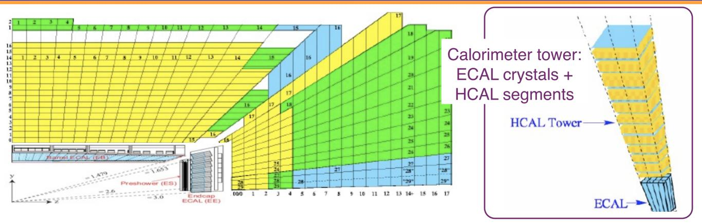
✦ Jets are reconstructed from energy depositions in the Electromagnetic and Hadron calorimeters, grouped in projective towers.
