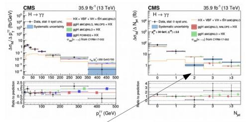
"Oscillating" behavior is typical for non-regularized unfolding, together with negative correlation coefficients
