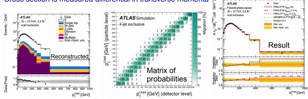
For each observable, the unfolding procedure starts from the number of events at reconstruction level in bin j of the distribution  $(N_{reco}^{j})$ , after subtracting the background events estimated as described in Section 5
