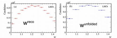
Figure 3: The spectra (a)  $dN_{\text{meas}}/dw$  before unfolding and (b)  $dN_u/dw$  after unfolding, for the decay  $\Lambda_b^0 \to \Lambda_c^+ \mu^- \overline{\nu}_{\mu}$ . The latter spectrum is then corrected for acceptance and reconstruction efficiency and fitted to the IW function  $\xi_B(w)$  with the procedure discussed in the text.
