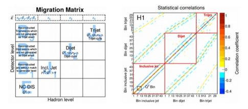
In this rather complex example, the data covariance includes non-diagonal elements (jets emerging from the same event are correlated). The matrix A has dimension of order 12000x3300. Only 10% (~320) of the unfolded bins are used for cross-sections, the other bins are nuisance parameters for control regions.
