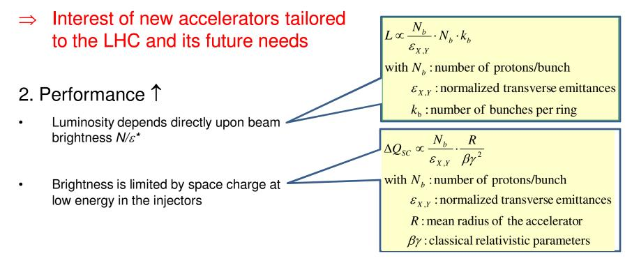
$\Rightarrow$  Need to increase the injection energy in the synchrotrons
