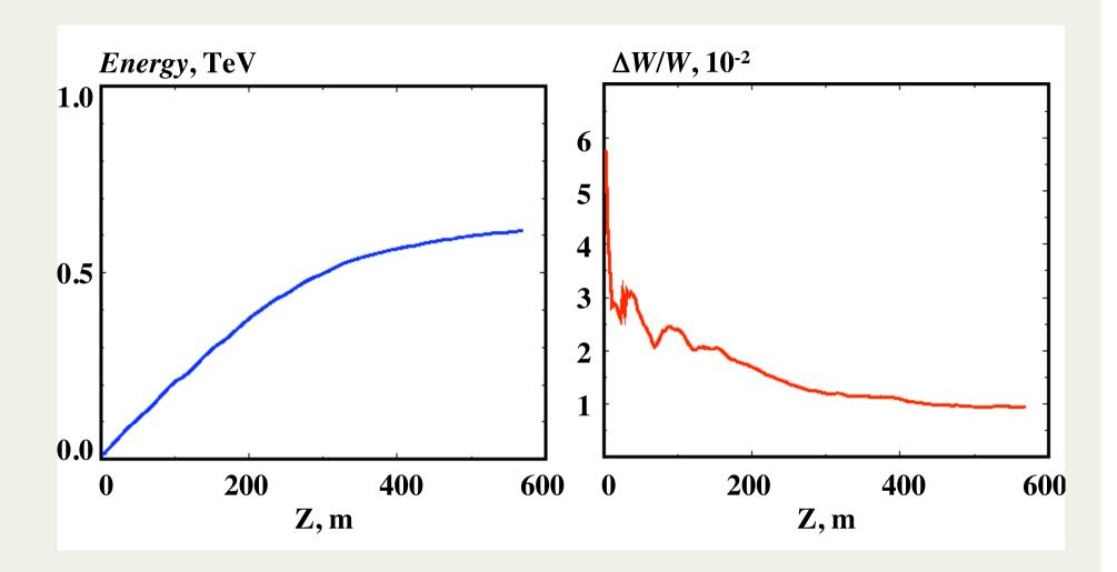
A Tevatron or HERA type proton beam, compressed to 100 microns but with 10% momentum spread, would allow to create a 600 GeV electron beam.
