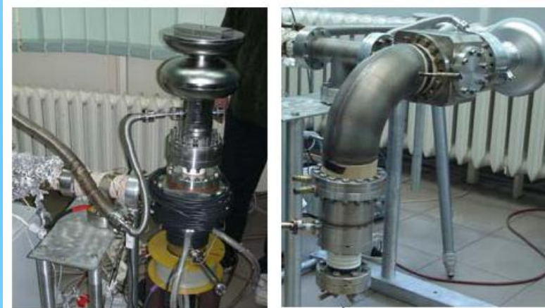
Location of the heater with lead stub for plasma formation
