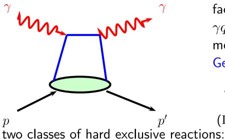
factorization in a hard subprocess, e.g.  $\gamma q \rightarrow \gamma q$ , and a soft proton matrix element, parameterized as a General Parton Distribution
