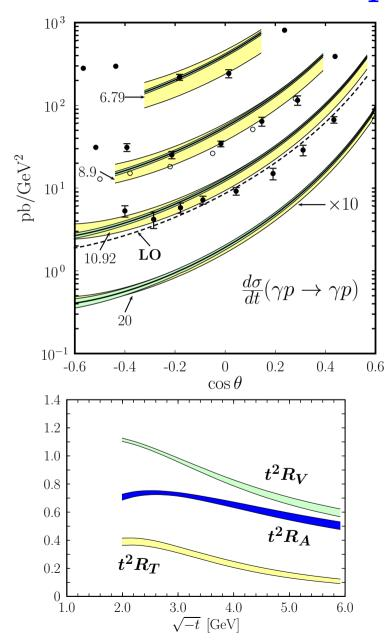
$$\frac{d\sigma}{dt} = \frac{d\hat{\sigma}}{dt} \left\{ \frac{1}{2} \frac{(s-u)^2}{s^2 + u^2} \left[ R_V^2(t) + \frac{-t}{4m^2} R_T^2(t) \right] + \frac{1}{2} \frac{t^2}{s^2 + u^2} R_A^2(t) \right\} + \mathcal{O}(\alpha_s)$$
