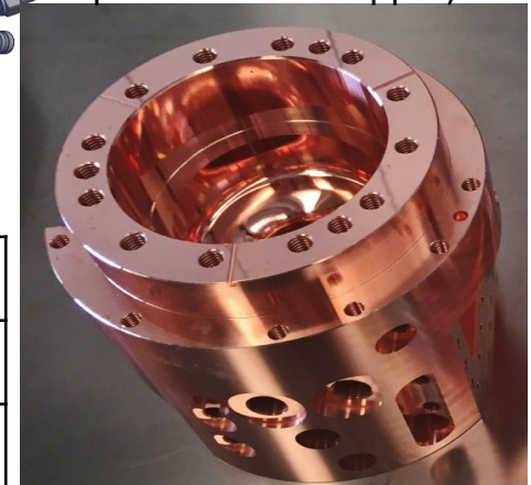
Body of the gun (single piece of OFHC copper)
