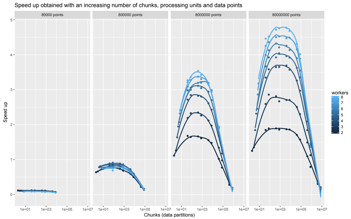
Figure 8: Speed up obtained with TProcessExecutor for different sizes of the data and different number of chunks when benchmarking with the second dataset. The measures have been taken with different number of processing units
