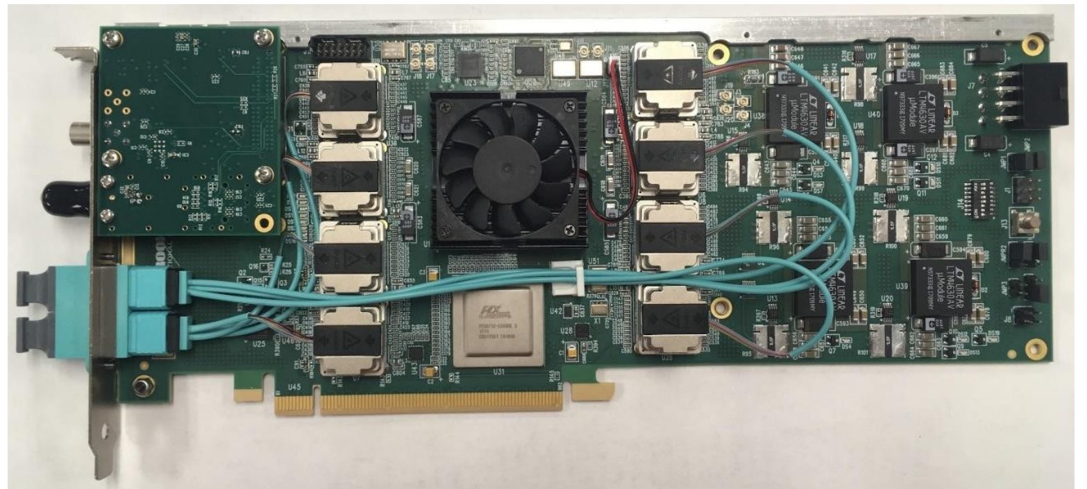
FLX-712 : ATLAS production board for Run 3
