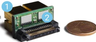
Fig. 2: 128 channel LabPET II detection module.
