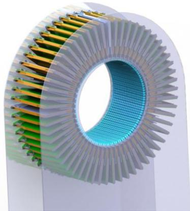
The UHR brain PET scanner combines **1,008 LabPET II detection modules** for a total of **129,024 individual channels**. The modules form a tube with a diameter of 390 mm and an axial length of 235 mm. This scanner can achieve a **spatial resolution of 1.3 mm**.
