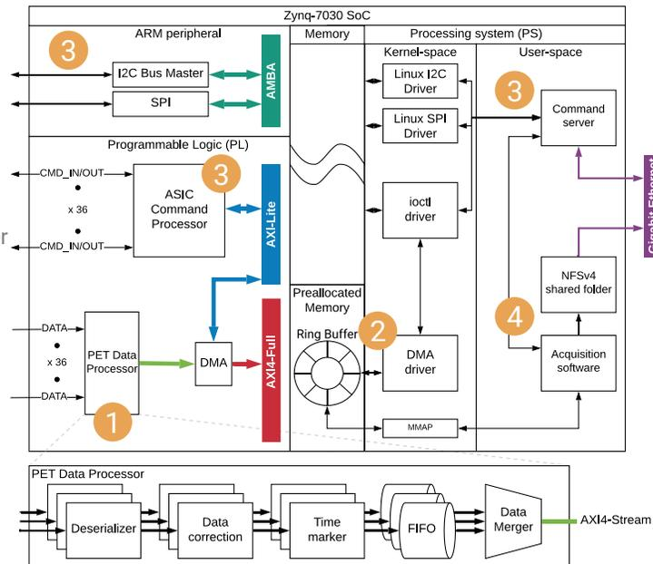
Fig. 5: Architecture of the embedded software for the UHR DAQ.
