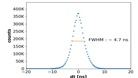
Fig. 7: Time resolution of two BrainDev in coincidence.
