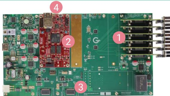
Fig. 4: BrainDev PCB: Proof of concept for the UHR data acquisition system based on a Xilinx Zynq-7020 and containing 12 LabPET II ASIC.
