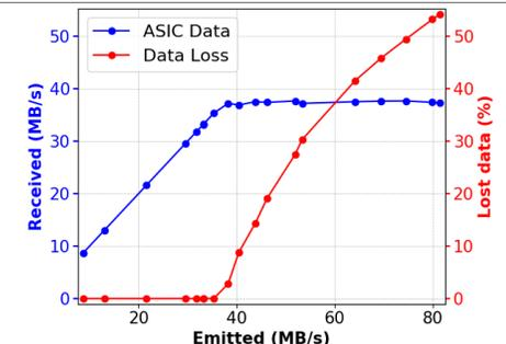
Fig. 6: Acquisition benchmark using the UHR DAQ.
