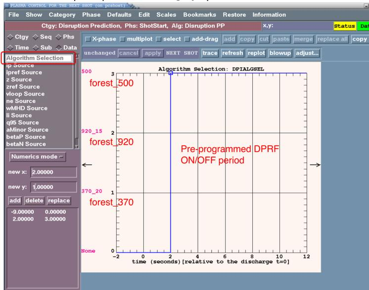
Four parameters need to be set before DPRF running with plasma discharge for real-time disruption warning:
