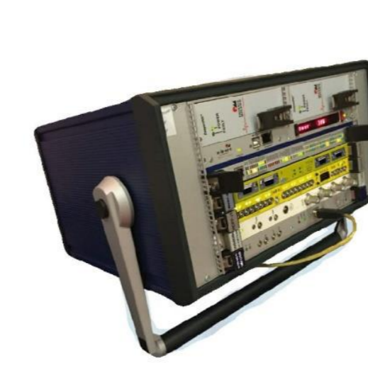
Portable VME-DAQ Mesytec Digital Pulse Processor
