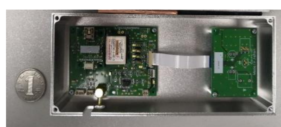
The different power driver circuit operating the same SiPM for the same photon signal
