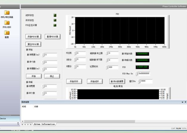
The environment for the user interface is determined to be Microsoft Windows. It can switch to different dialog views as needed by the user. The user can set the pulse width, the pulse numbers, the PID gain, etc.
