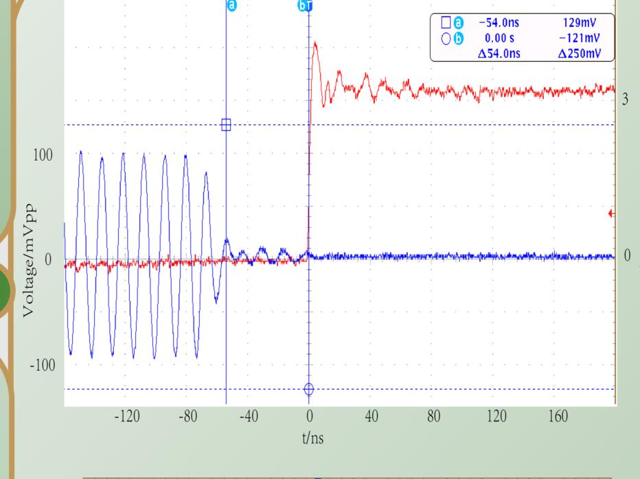
The spark detection is tested with 73 MHz signal. The latency of the circuit is less than 60 ns. With a higher frequency, the latency would be smaller.
