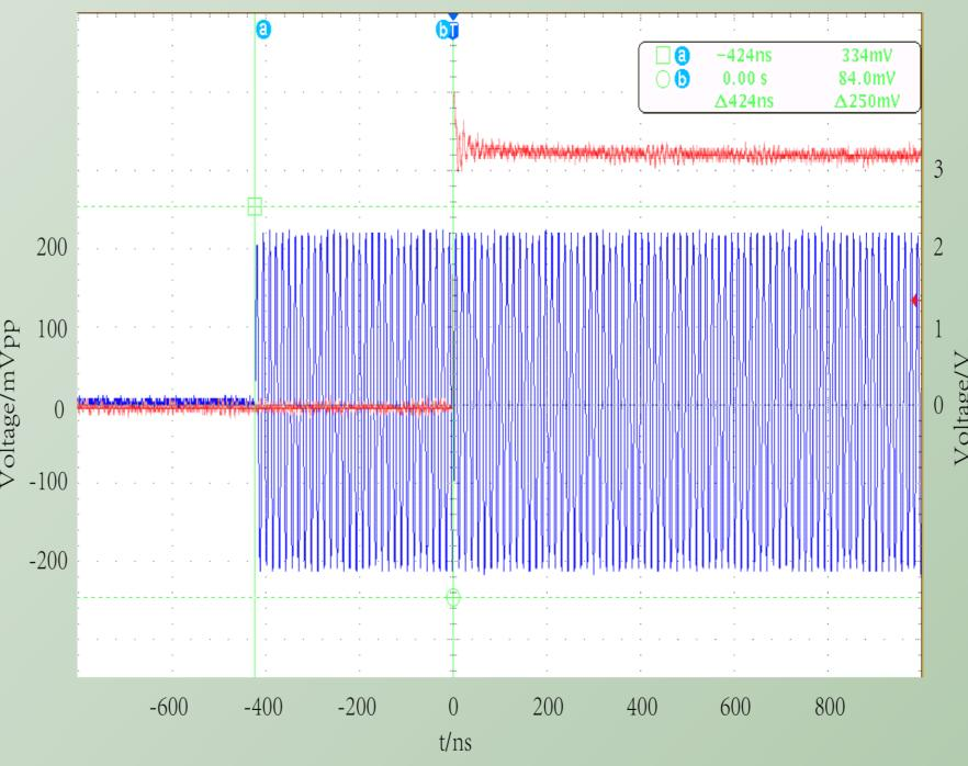
The reverse power detection is tested with step signal. The circuit work at 250 MHz frequency. The latency of the circuit irrelevant to the frequency of the signal.
