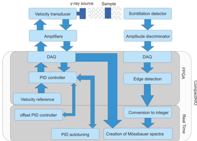
Fig. 3. Block diagram of program code of developed Mössbauer spectrometer.
