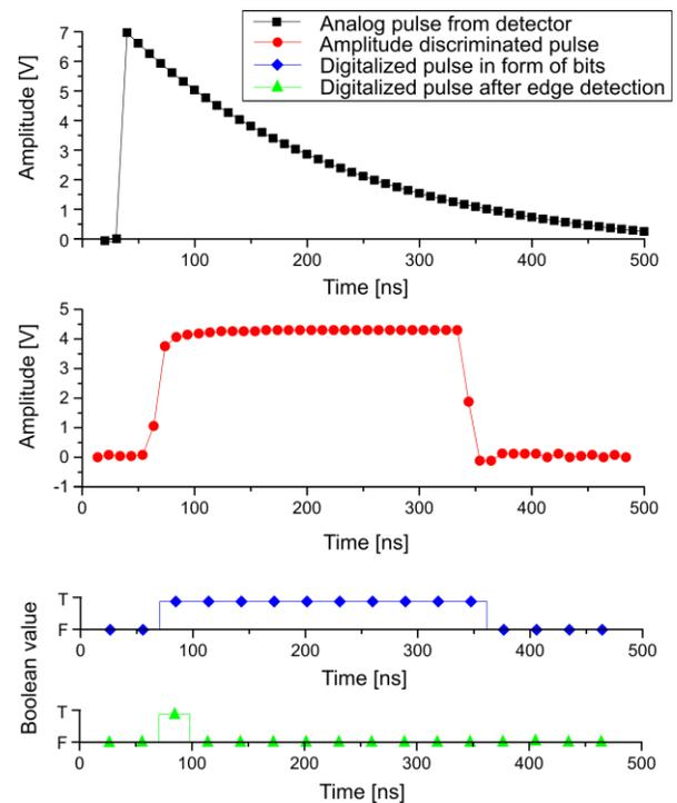
Fig. 4. Processing of signal from scintillation detector. Original signal from scintillation detector (a), signal after amplitude discrimination (b), Boolean representation of signal as an array in FPGA of CompactRIO (c), Boolean representation of valid detections of gamma rays after edge detection (d).
