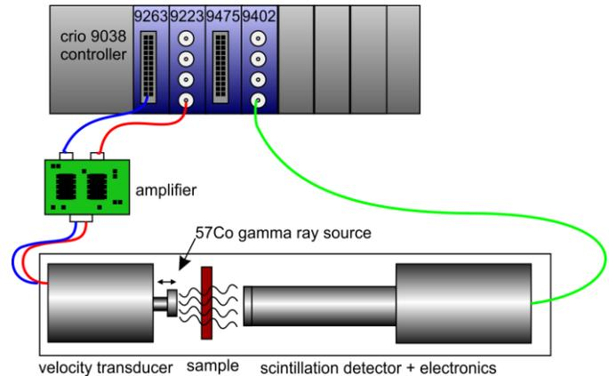
Fig. 1. Wiring scheme of developed spectrometer
