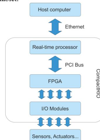
Fig. 2. CompactRIO architecture.
