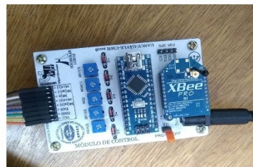
Fig. 3. Wireless transmission with Xbee module.
