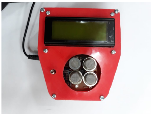
Fig. 2. Finished module with MQ4-1, MQ4-2, MQ5 and MQ9 gas sensors.
